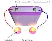
When electric current is able to flow around a complete circuit it can be used by electrical appliances, such as light bulbs.
